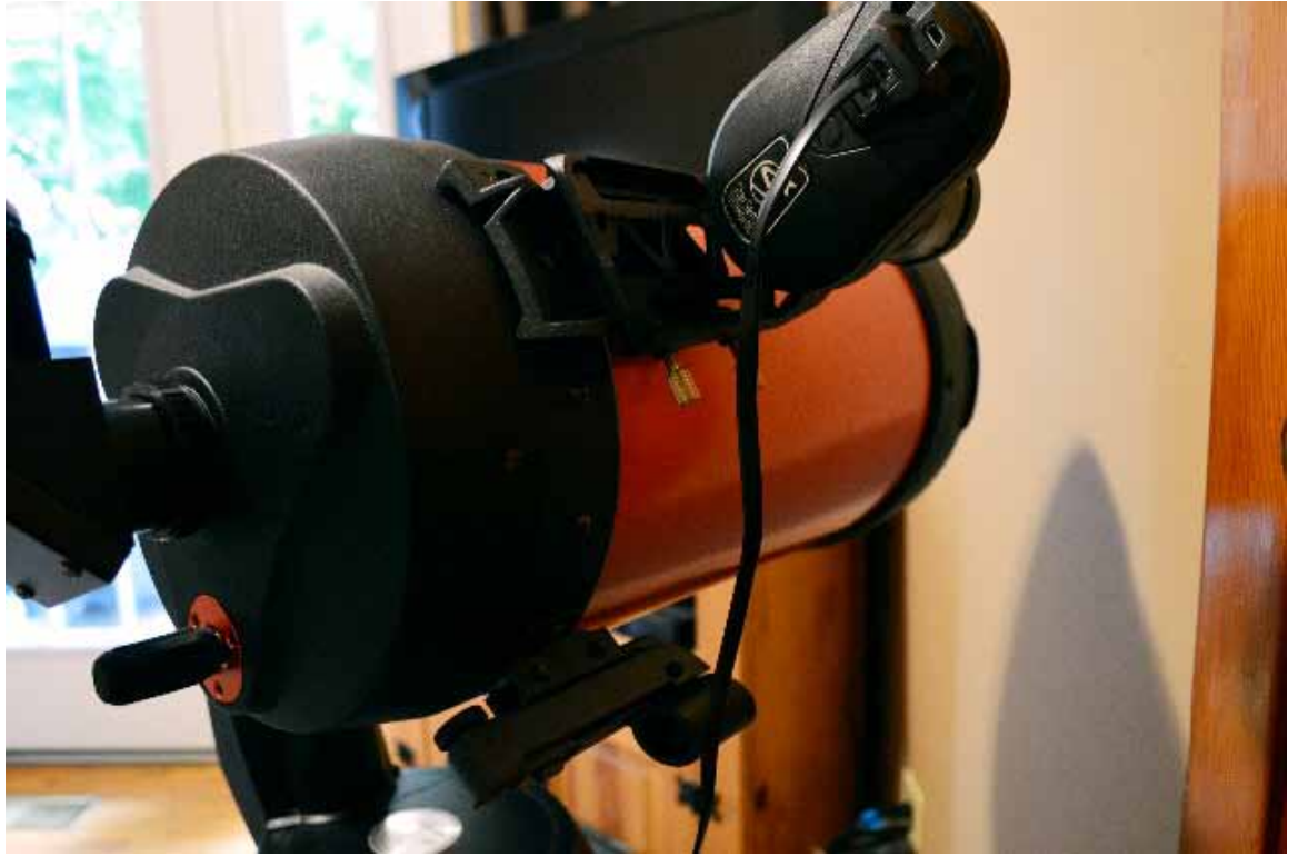
Celestron StarSense AutoAlign accessory mounted on Paul Ward's Celestron SE8. Photo by Paul Ward.
